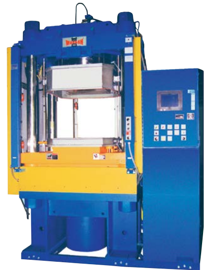
MiniViewpoint with PanelView C600 Operator Interface Mid-level control system for proportional control pressure and for integral temperature control.
